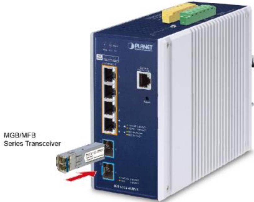
Figure 2-19: Plugging in the SFP/SFP+ Transceiver
