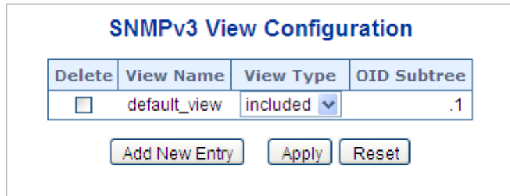
Figure 4-2-2-10: SNMPv3 Views Configuration Page Screenshot
